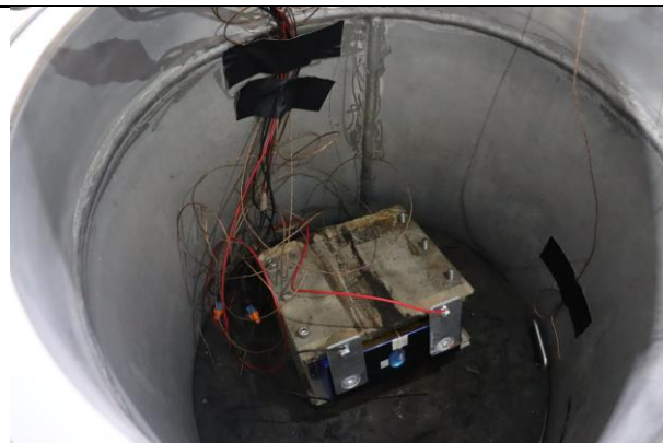
Figure 25: Sample 5 instrumented and inside gas test chamber
