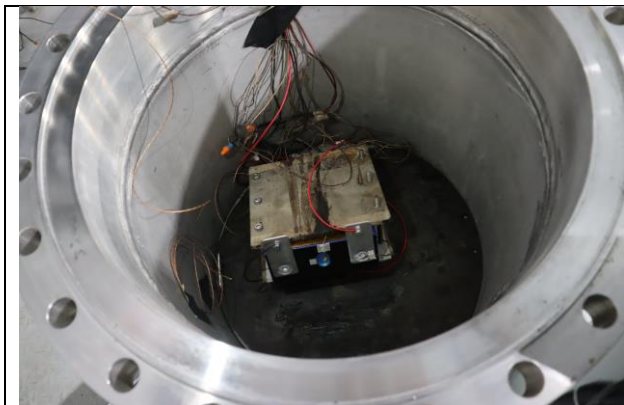
Figure 25: Sample 5 instrumented and inside gas test chamber
